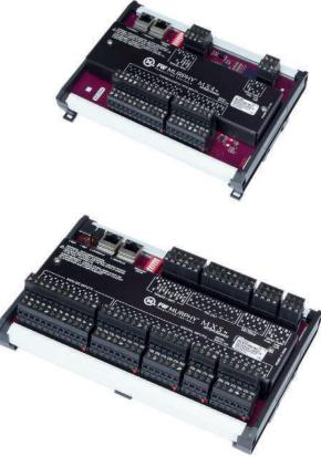
•Operating temperature: -40° to 185° F (-40° to 85° C) • Power input: 11 W max 10-30 VDC
