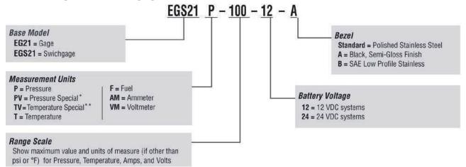
NOTE: EG21 and EGS21 are designed for use with 12-volt systems. For 24-volt systems, voltage reducing resistors are included in the wire/connector assembly. No designator required for Standard configurations.
