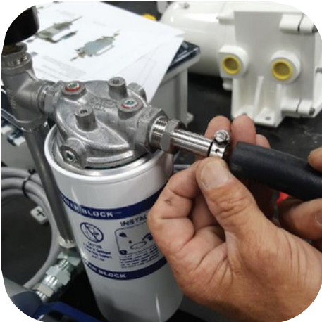
Step 4: Attach the black discharge hose to the fine filter with clamp
