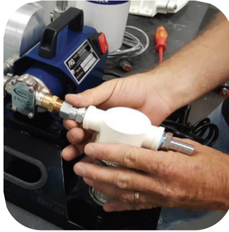
Step 2: Attach the strainer assembly (male to female connection)
