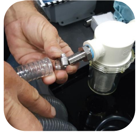
Step 3: Attach the clear suction hose to the strainer with clamp
