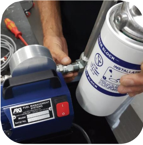
Step 1: Attach the fine filter assembly (male to female connection)
